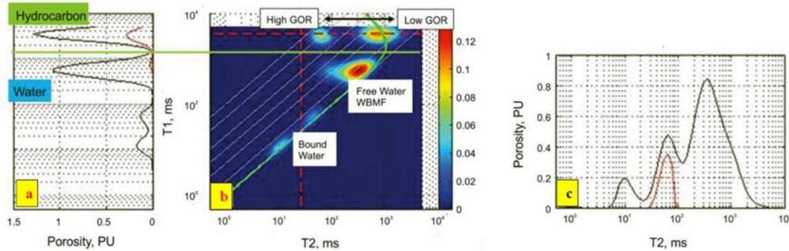
**Figure 6 2D NMR in the presence of WBM [3]**
