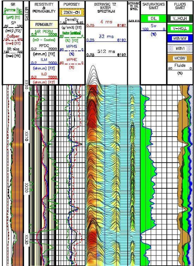
Figure 3 SIMET log display output from [1]
