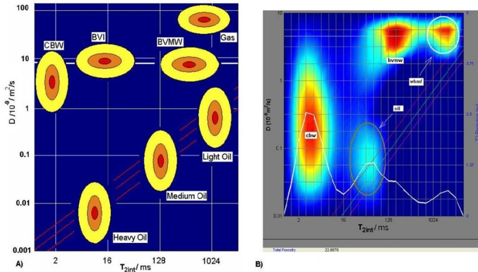
**Figure 4 A) schematic D-T2 map and B) Real data derived D-T2int showing heavy oil spot, clay bound water (cbw), movable water volume (bvmw) and water based mud filtrate (wbmf) from [1].**
