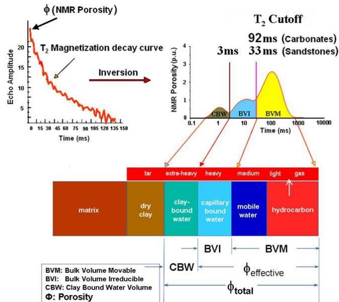
Figure 1 1D-NMR porosity model: Cut-off partition of  $T_2$  spectrum
