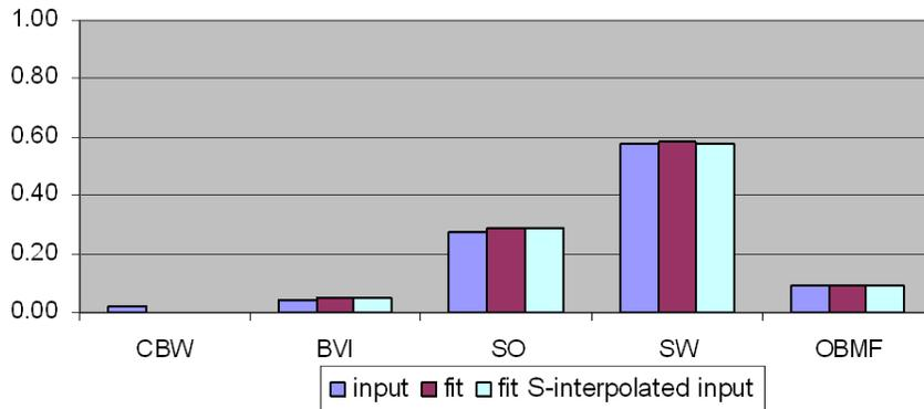
**Figure 10 Volumetric results of fitting a T2 distribution containing oil and movable water.**
