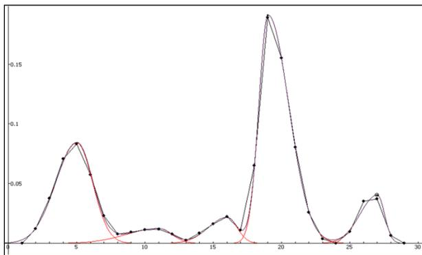
**Figure 9 Fitting of T2 components of a reservoir layer containing oil saturation and also movable water. Depth x3.**
