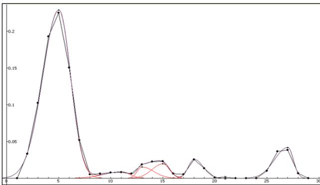
**Figure 7 Fitting T2 components of a reservoir layer at Swi. Depth x2.**
